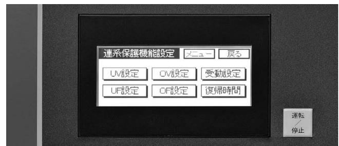
Fig. 6: Utility protective function setting screen of the “SANUPS P83E” touch panel
