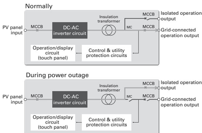
Fig. 2: A block diagram of an isolated operation circuit
