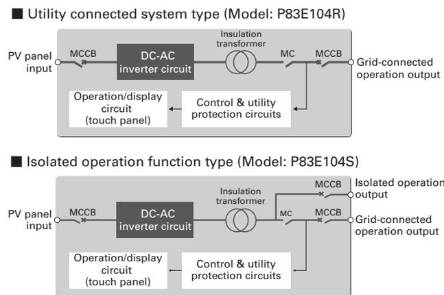
Fig. 4: Circuit block diagram of the “SANUPS P83E”
